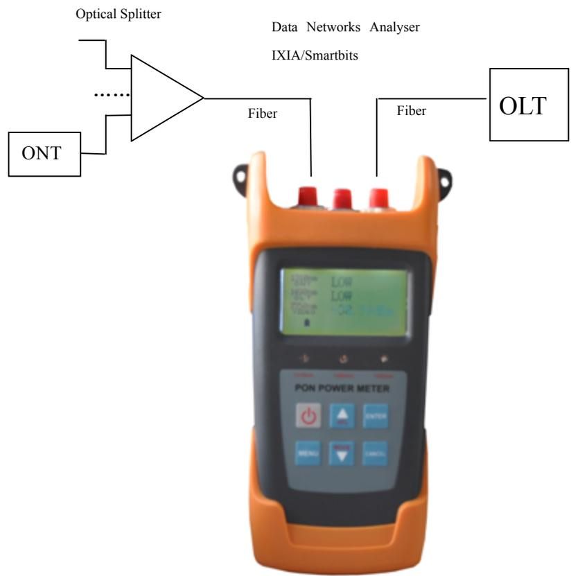
OLT PON Interface optical power test configuration diagram
